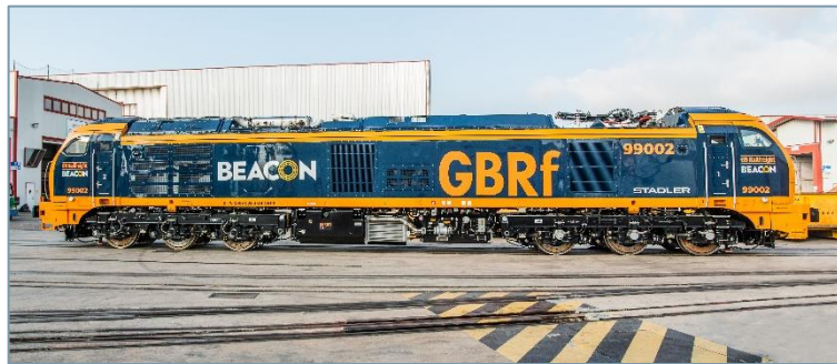
Bimodal locomotive for flexible freight transport
